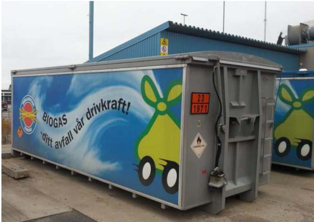
Container for transport of compressed vehicel gas (in gas cylinders) in Sweden Source: Thrän et al, 2014
